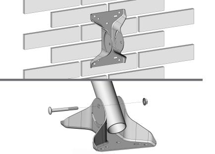
Install the pole to the base using pivot bolt
