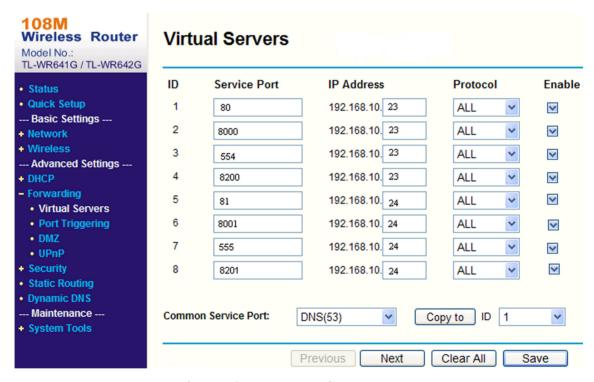
Figure 10-1 Port Mapping on Router
