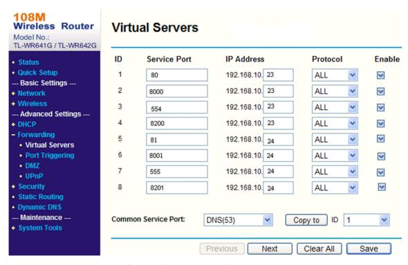
Figure 10-1 Port Mapping on Router
