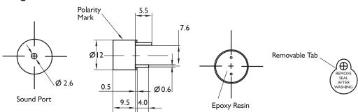
Dimensions : Millimetres Tolerance : ±0.5mm
