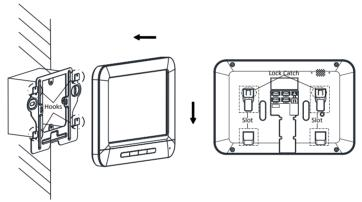
Figure 4-3 Hooking the Indoor Station to the Plate
