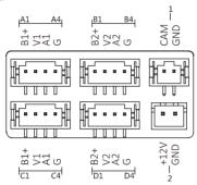
Figure 3-1 Terminals of Indoor Station
