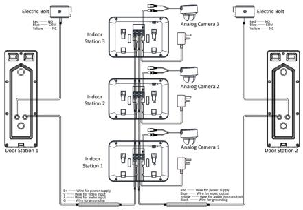
Figure 3-5 Wiring 3 (2 Door Stations and 3 Indoor Stations)
