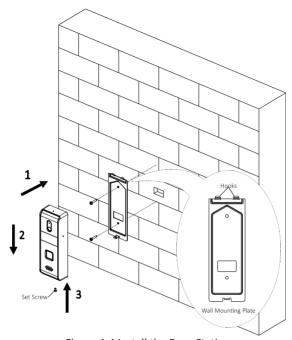
Figure 4-4 Install the Door Station
