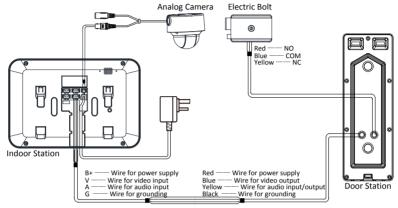
Figure 3-3 Wiring 1 (1 Door Station and 1 Indoor Station)
