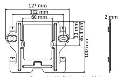
Figure 4-1 Wall Mounting Plate
