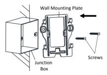
Figure 4-2 Installing the Plate
