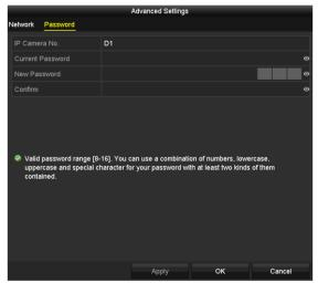
Figure 2-10 Password Configuration of the Camera
