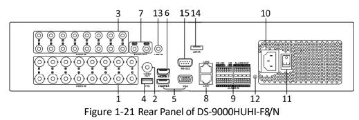
The rear panel of DS-9004HUHI-F8/N and DS-9008HUHI-F8/N provide 4 and 8 video input interfaces respectively.
