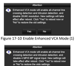
Figure 17-11 Enable Enhanced VCA Mode (2)
