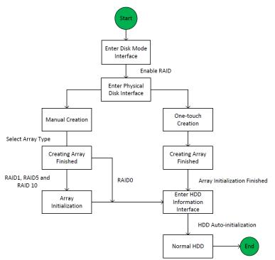
Figure 13-1 RAID Working Flow
