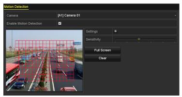
Figure 5-15 Motion Detection- Mask
