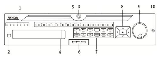
Figure 1-7 Front Panel of DS-9000HUHI-F8/N
