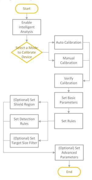
Figure 5-1 Flow Chart of Perimeter Protection Configuration
