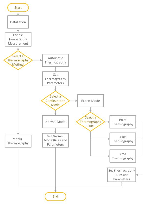
Figure 3-1 Thermography Configuration Flow Chart
