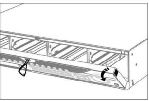
**Figure 1-6 Open Front Panel**
