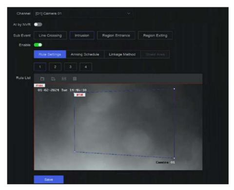
**Figure 13-2 Intrusion Detection**
