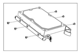
Figure 1-5 Fix Mounting Ears to HDD
