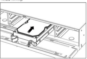
Figure 1-7 Insert HDD
