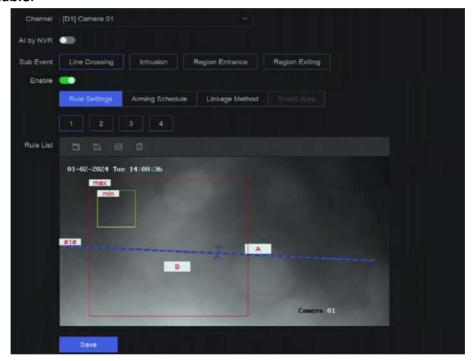
Figure 13-1 Line Crossing Detection
