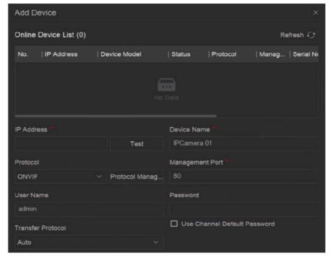
**Figure 6-2 Add Network Camera Manually**
