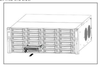
Figure 1-9 Push HDD Case into Slot
