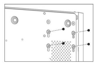
Figure 1-12 Fix HDD to Device Bottom
