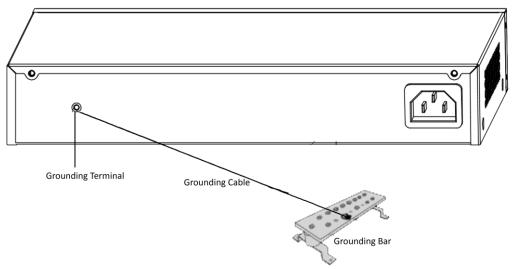
Figure 2-3 Grounding with Grounding Bar
