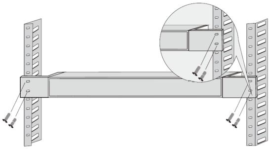
Figure 2-2 Fix Switch to Rack
