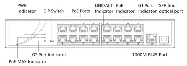
Figure 1-1 DS-3E0318P-E/M(B) Front Panel
