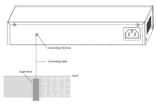
Figure 2-4 Grounding with Angle Steel
