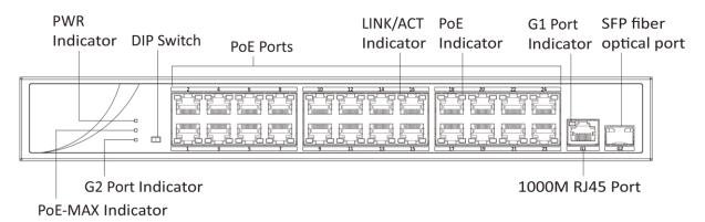
Figure 1-2 DS-3E0326P-E/M(B) Front Panel
