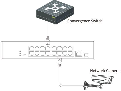
Figure 3-1 RJ45 Port Connection
