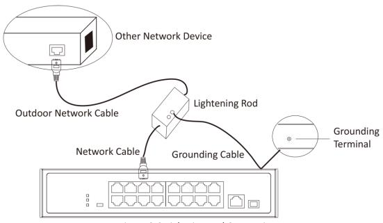
Figure 3-2 Lightning Rod Connection
