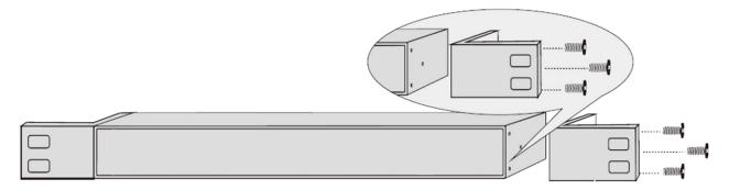
Figure 2-1 Install L-Shaped Brackets
