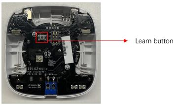
2. Hold down the button, after red light flash 3 times, means reset successfully, as below
