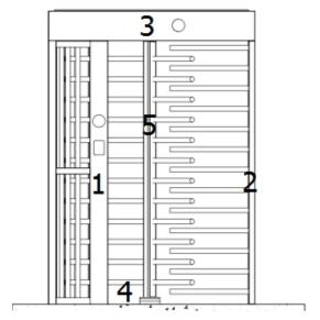
Assemble both sides of guardrail 1 part and 2 part firstly. Then place the 3 part top upper box over the 1 part and 2 part and tighten the mounting screws; lay 4 part bearing mechanism at the bottom of a rotating shaft; Install 5 part rotation, tighten the top mounting screws; Check the verticality of the shaft. Adjust and check the level and vertical of the machine.
