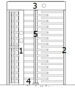
Assemble both sides of guardrail 1 part and 2 part firstly. Then place the 3 part top upper box over the 1part and 2 part and tighten the mounting screws; lay 4 part bearing mechanism at the bottom of a rotating shaft; Install 5 part rotation, tighten the top mounting screws; Check the verticality of the shaft. Adjust and check the level and vertical of the machine.
