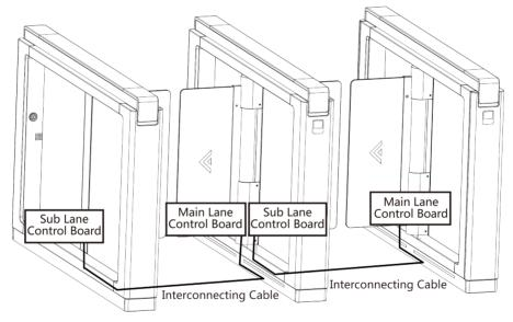
Figure 5-4 Connect Interconnecting Cable
