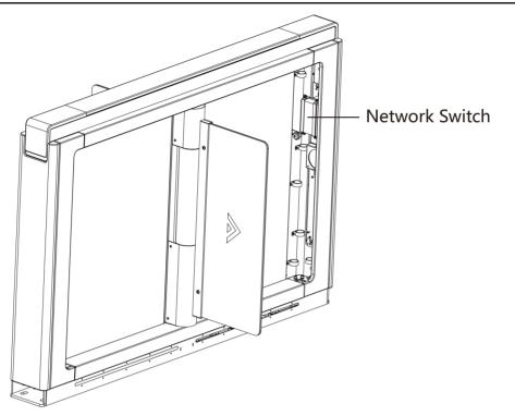
**Figure 5-5 Network Switch Position**
