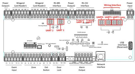
Figure 5-10 Access Control Board
