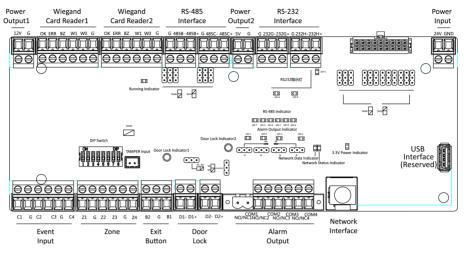
**Figure 5-9 Access Control Board**
