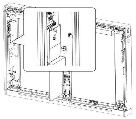
Figure 5-6 Face Recognition Terminal Power Supply Wiring Position
