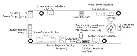
Figure 5-7 Main Control Board
