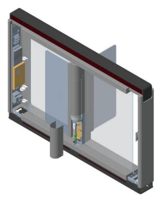
Figure 3-7 Remove Motor Bottom Cover
