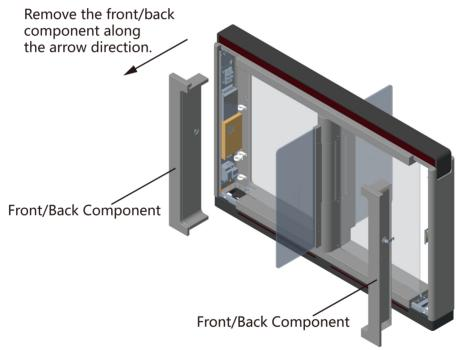
Figure 4-3 Remove Components
