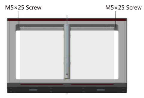
Figure 4-7 M5×25 Screws Position
