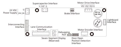
Figure 5-8 Sub Control Board
