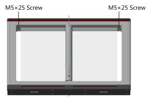
Figure 4-2 M5×25 Screws Position
