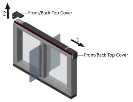
Figure 4-11 Remove Front and Back Top Cover
