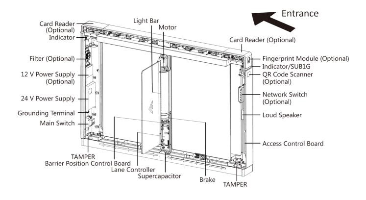
Figure 5-1 Components Diagram
