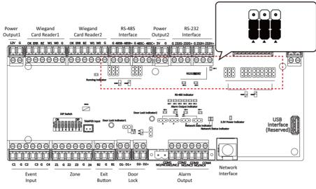
Figure 6-2 Jumper Cap Status of RS-485 Interface
