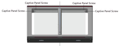
Figure 4-10 Loosen Captive Panel Screw
