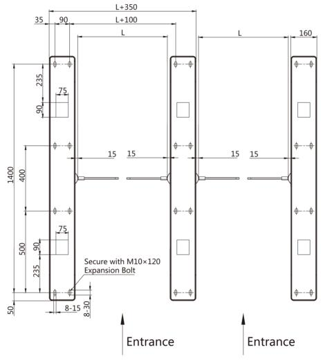
Figure 3-11 Installation Footprint
