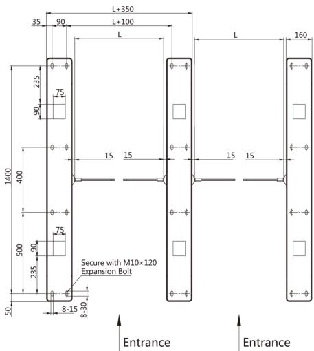
Figure 2-1 Hole Position Diagram
