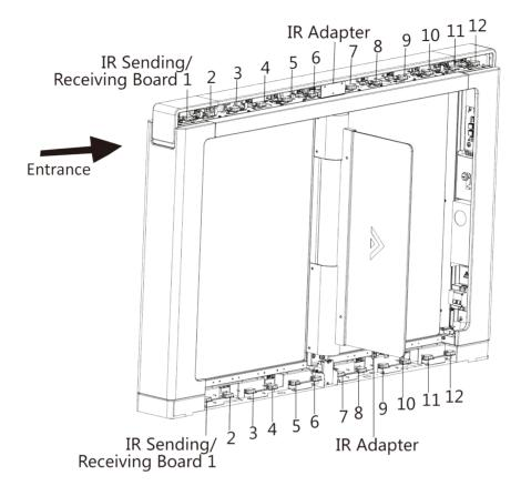
Figure 5-2 IR Sending/Receiving Module Position
