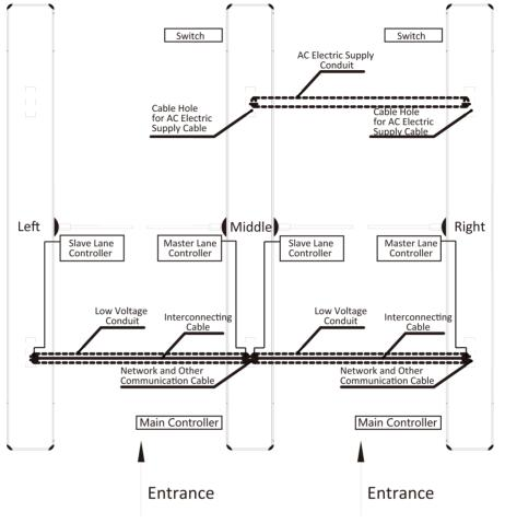
Figure 2-2 System Wiring Diagram (General Wiring)
