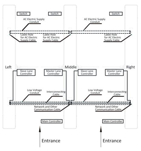
Figure 2-3 Wire Face Recognition Terminal
