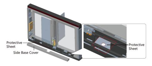
Figure 3-9 Disassemble Two Protective Sheets
