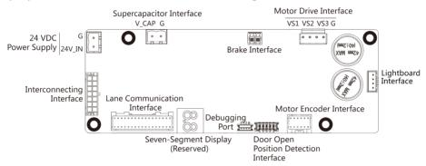
**Figure 5-8 Sub Control Board**
