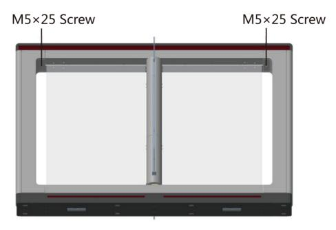
Figure 4-7 M5×25 Screws Position
