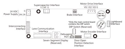
**Figure 5-7 Main Control Board**
