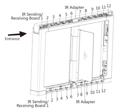
Figure 5-2 IR Sending/Receiving Module Position
