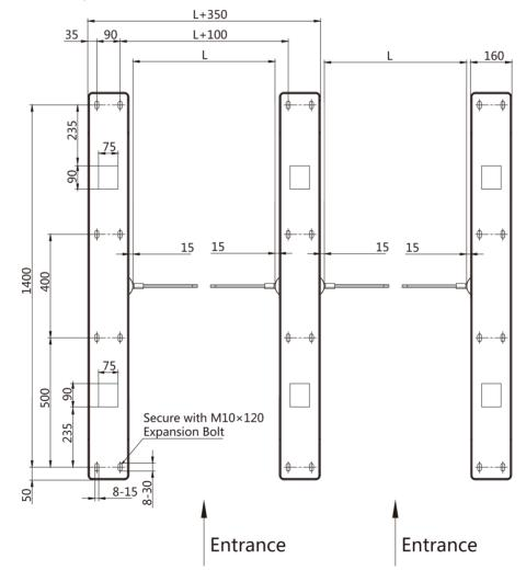
**Figure 3-11 Installation Footprint**
