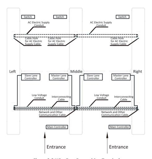
Figure 2-3 Wire Face Recognition Terminal
