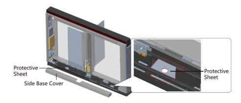
**Figure 3-9 Disassemble Two Protective Sheets**
