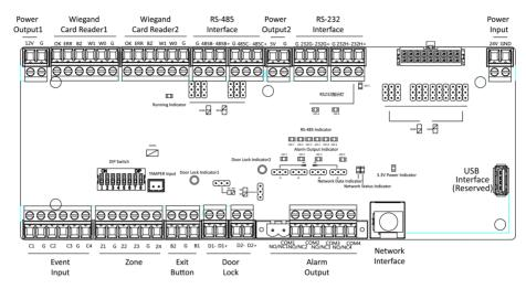
**Figure 5-9 Access Control Board**
