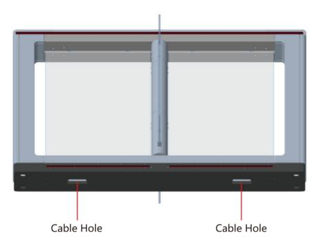
Figure 5-3 Cable Hole of Interconnecting Cable
