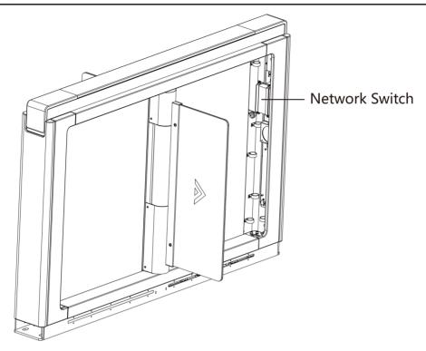
**Figure 5-5 Network Switch Position**
