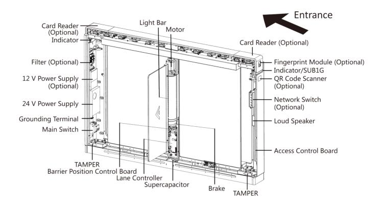
Figure 5-1 Components Diagram
