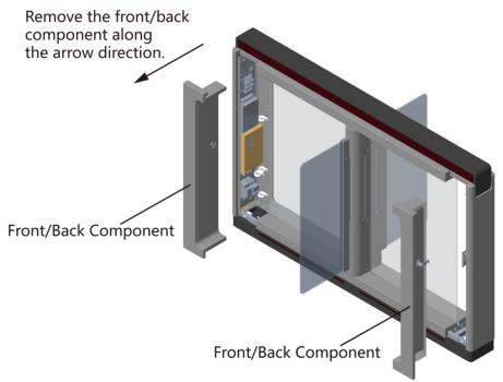
**Figure 4-8 Remove Components**
