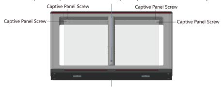
Figure 4-10 Loosen Captive Panel Screw
