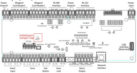
Figure 6-1 Initialization Jumper Cap
