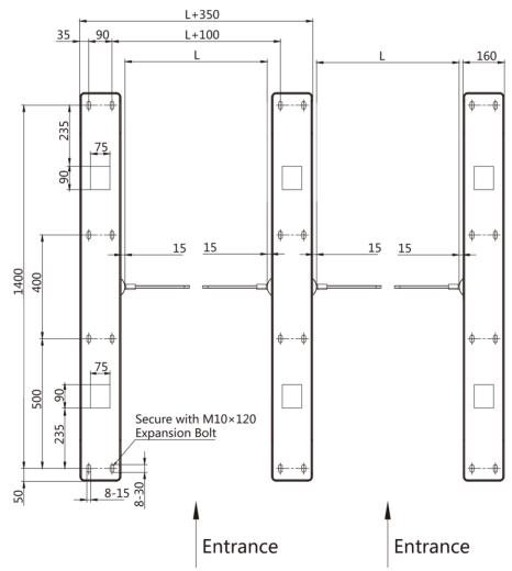
Figure 2-1 Hole Position Diagram
