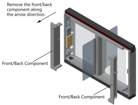
**Figure 4-3 Remove Components**
