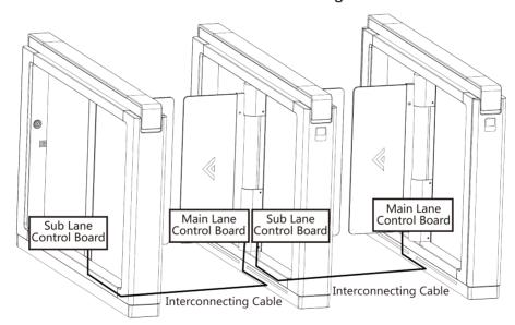
**Figure 5-4 Connect Interconnecting Cable**
