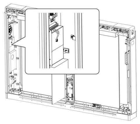
Figure 5-6 Face Recognition Terminal Power Supply Wiring Position
