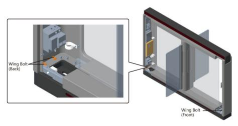
Figure 3-4 Loosen Wing Bolt
