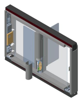
**Figure 3-7 Remove Motor Bottom Cover**
