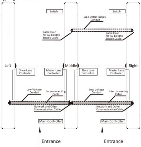
Figure 2-2 System Wiring Diagram (General Wiring)
