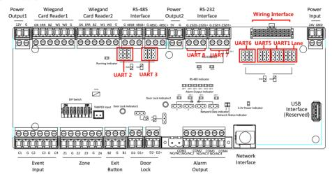
Figure 5-10 Access Control Board
