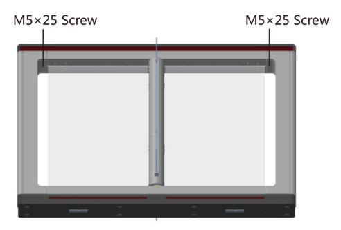
Figure 4-2 M5×25 Screws Position
