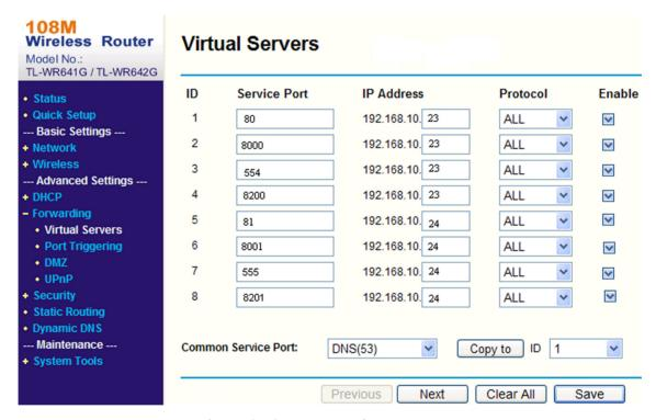
Figure 2-13 Port Mapping on Router
