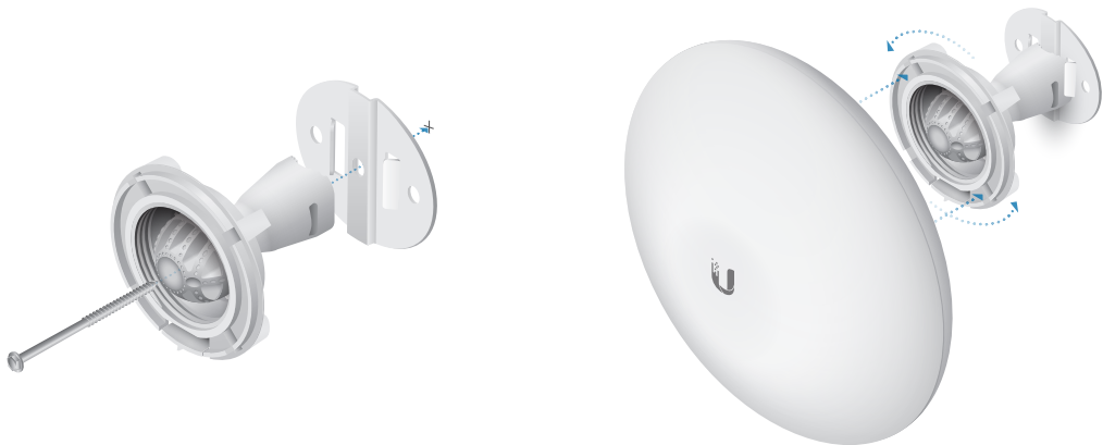
Installation Using the NanoBeam Wall Mount Kit
