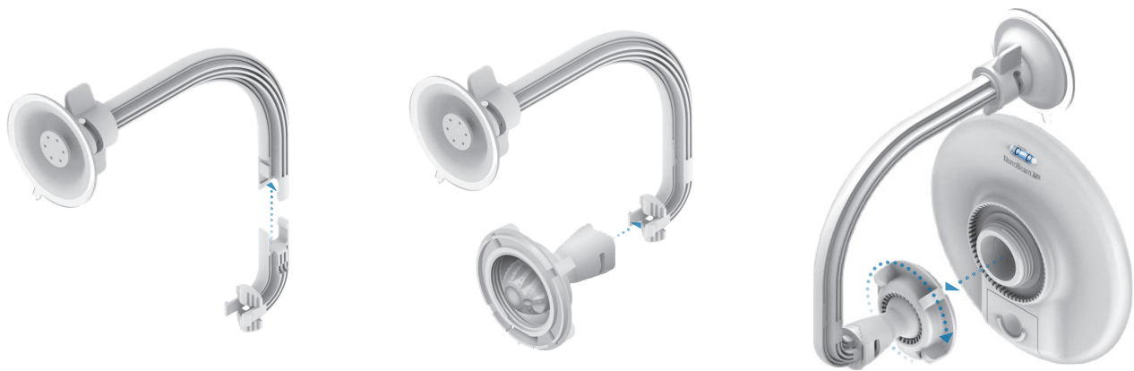
Installation Using the NanoBeam Window Mount
