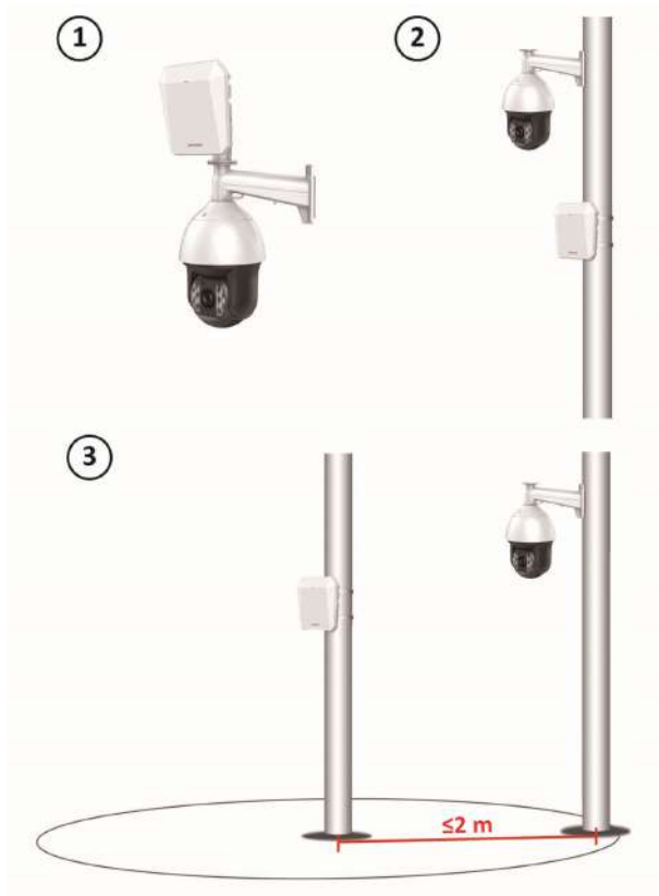
Figure 5-5 Installation Scene for One Point Calibration
