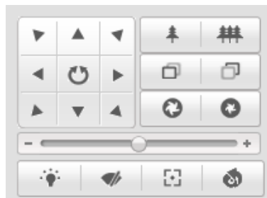
Figure 6-3 PTZ Control Panel
